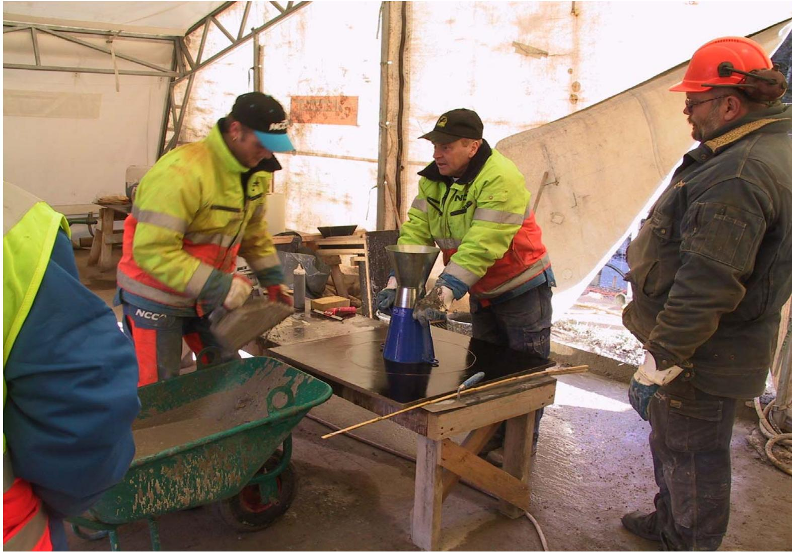
Slump-flow test of Self Compacting Concrete
